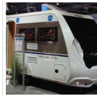
Vision Systems' electronically dimmable windows, using Research Frontiers' SPD-SmartGlass technology, on (at left) a Knaus caravan, and a LCI demonstrator (at right).
