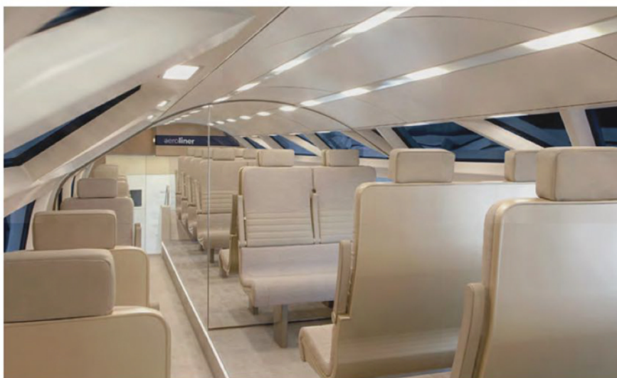
Upper deck: the curvature of the upper level of the vehicle to accommodate the UK loading gauge limits the seat layout to 2+1. The mirror on the mock-up gives the impression of a full-length vehicle.
