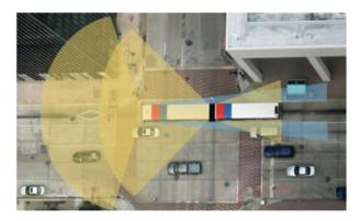
First up is Smart-Vision, which is a camera monitoring system that replaces rearview mirrors with high-definition cameras and interior displays. Developed by Vision Systems' business unit Safety Tech, Smart-Vision is an efficient solution for buses, coaches and recreational vehicles, providing optimised visibility and enhanced ergonomics.
