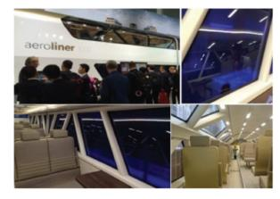
At 2016 InnoTrans, a full-scale mockup of the AeroLiner3000, with Vision Systems Nuance brand of SPD-Smart EDWs (Electronically Dimmable Windows) – shown in a darkly tinted state at top right and bottom left – was exhibited at the booth of the German Aerospace Centre (DLR).
